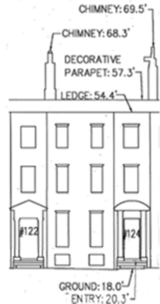
Two-Dimensional CAD Deliverable from Laser Scan
